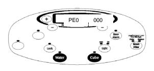
**NOTE:** If the Program CODE is correct, the Programming Mode is exited by pressing Door Alarm Keypad for 3 seconds.
