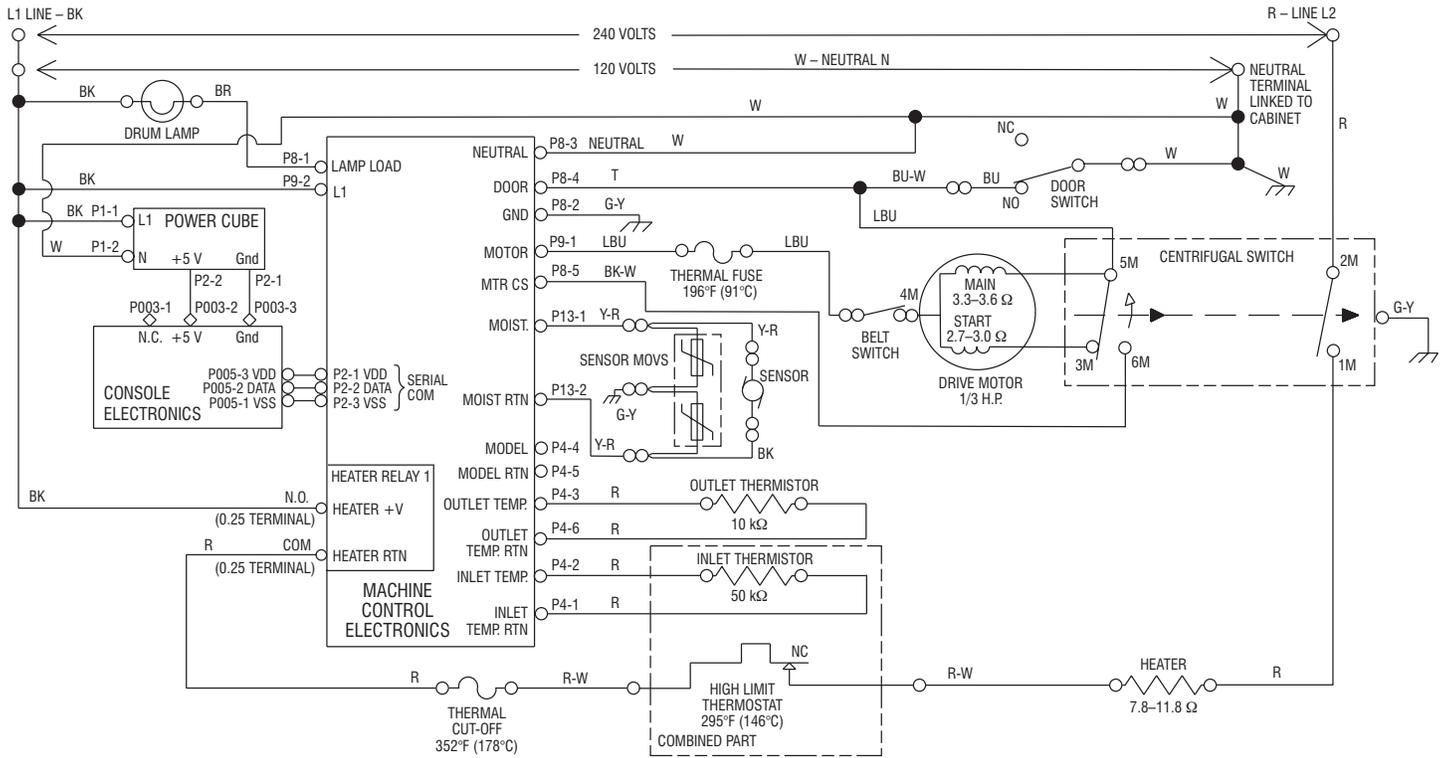
**GAS DRYER WIRING DIAGRAM**
