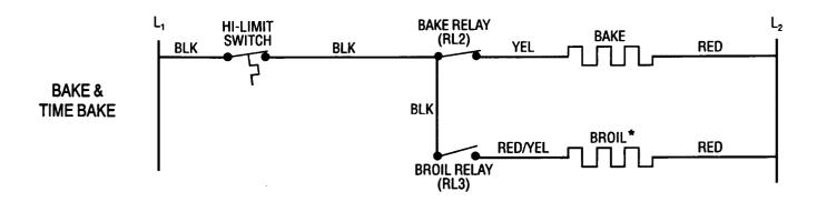
\* Broil element is on approximately 8% of the time during BAKE mode. RL2 and RL3 relays will be on at the same time. During first (pre-heat) cycle, only the Bake element is on.
