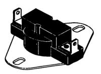
The high limit switch is a normally closed single pole, single throw switch with an opening temperature of approximately 225° F. The switch is attached to the top insulation retainer, in front of the fan.
