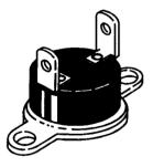
The unit is equipped with a fan disc switch (blower switch). The switch is a normally open single pole, single throw switch that closes at 160° F and opens at 145° F. The switch is located on the top insulation retainer, midway between the fan and clock.
